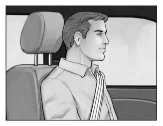
Adjust your head restraint so that the top of the restraint is closest to the top of your head. This position reduces the chance of a neck injury in a crash. Pull straight up on the head restraint to raise it and push it down to lower it.
